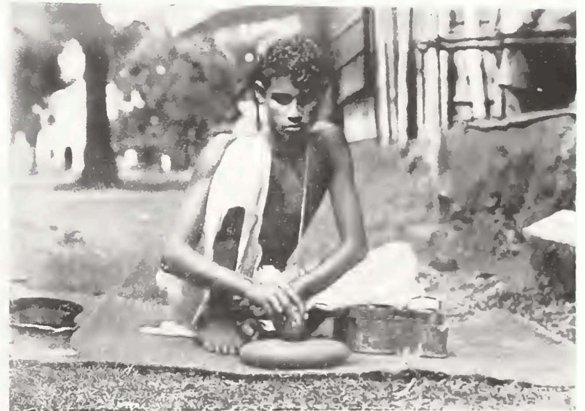
FIG. 10. RUBBING DOWN CINNABAR (HINGOL) TO COLOUR LACQUER RED. DINAJPUR.
