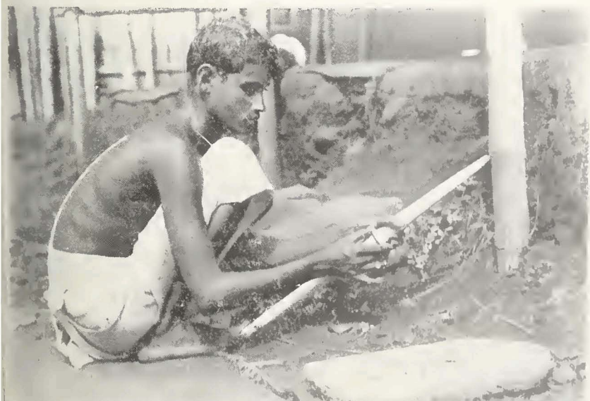
FIG 6. RUBBING DOWN THE INNER SURFACE OF A CHANK WORKING SECTION. DINAJPUR.
